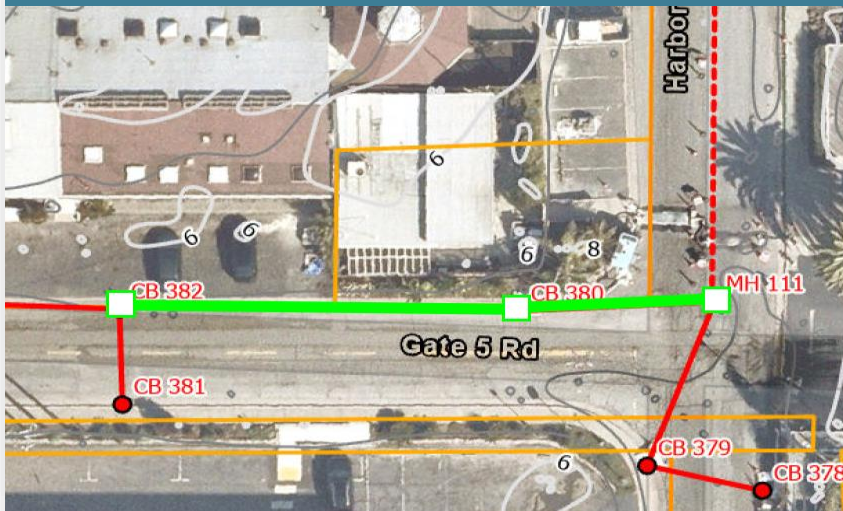
Storm Drain System at Harbor & Gate 5 Road
